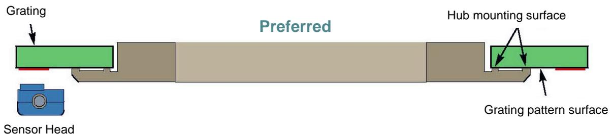
The illustration above shows the recommended orientation of grating and the hub where the grating's pattern surface is contacting the hub's mounting surface.
