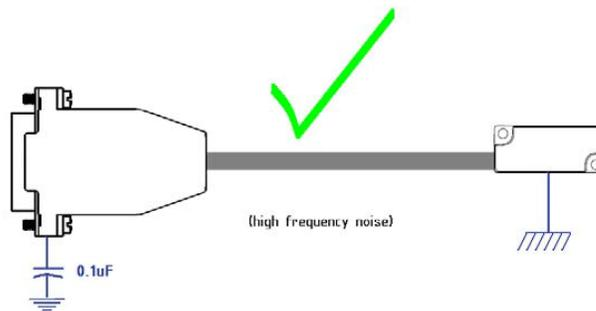
In this example, the capacitor will act as an open circuit for low frequency noise (or a DC potential between grounds) and a short circuit for higher frequencies. This technique is highly recommended for applications where high frequency interference is common.
