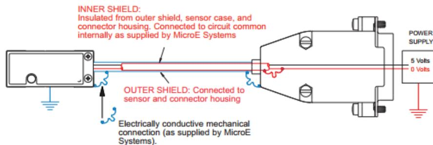
Sensor mounted to poorly grounded or non-conducting surface:
