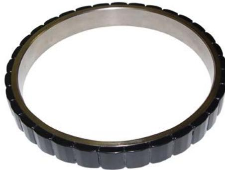
*Figure 1a: A Celera Motion Omni™ Series direct drive low profile rotor. The magnets are bonded to the surface of the rotor hub ring. This example has 32 poles and the magnets are shaped on the surface to minimize cogging torque.*
