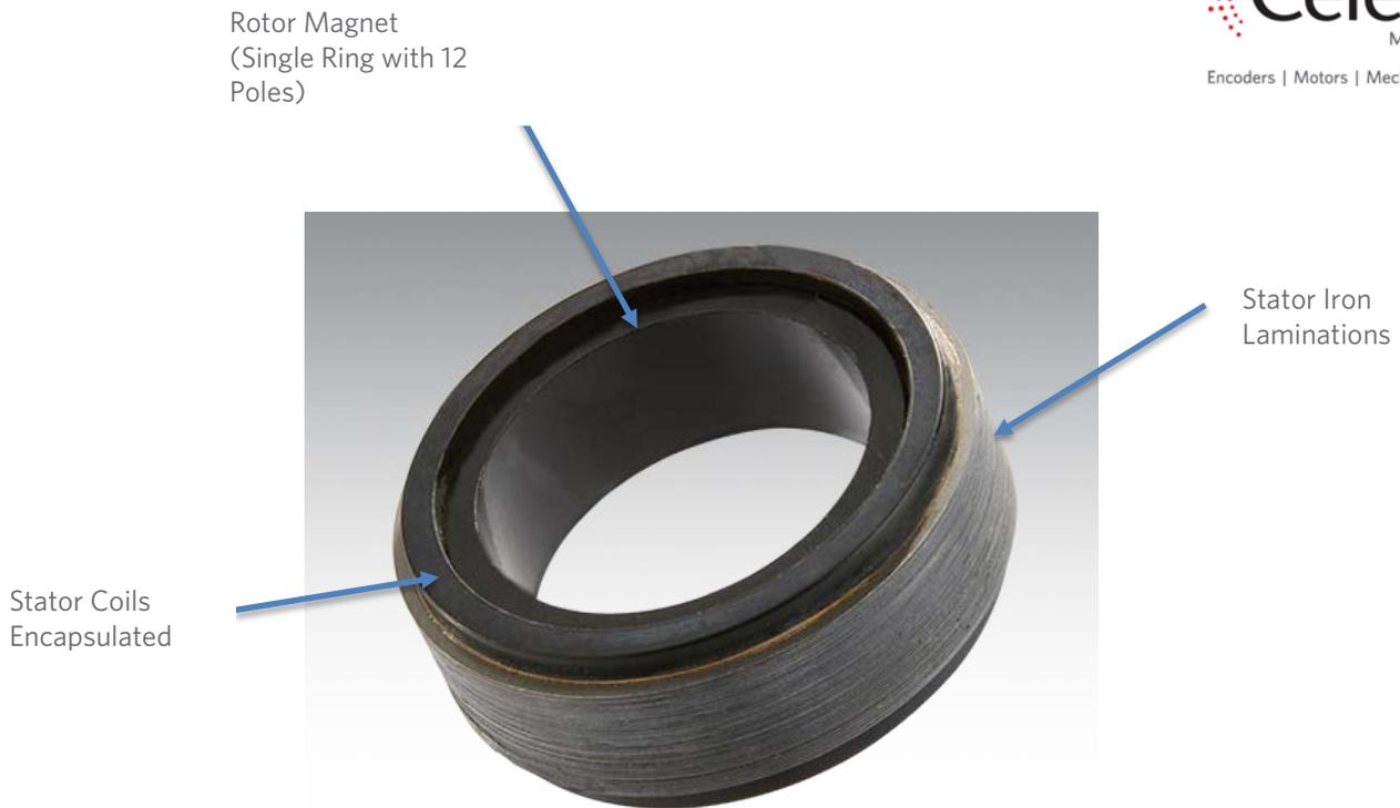
Figure 3b: The rotor in the center is a single piece ring magnet with 12 poles.
