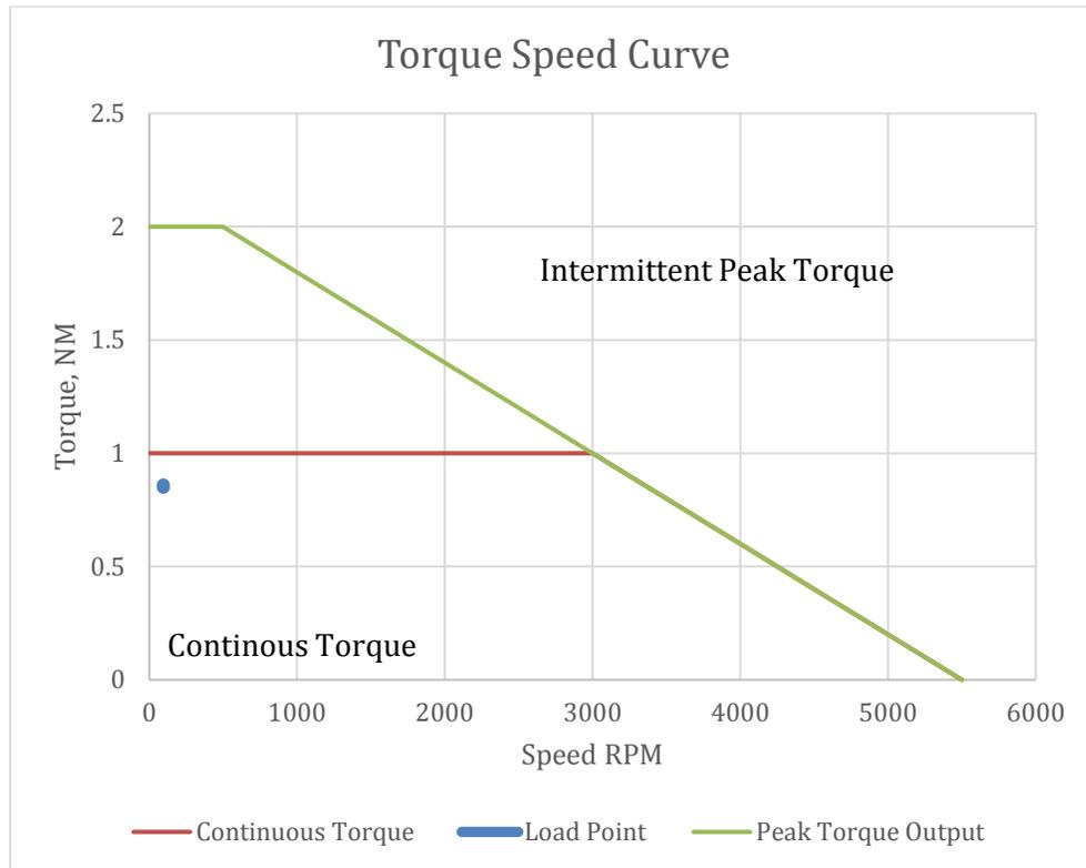
Figure 4 adds the green data line to the plot showing a higher torque limit. This peak torque output requires additional current and comes at the expense of extra heating so it can only be used intermittently with a duty cycle. Notice that allowing for higher current only improves torque at lower speeds. The torque output at higher speeds is governed by the available voltage and the motor winding resistance. To produce more torque at higher speeds the voltage must be higher.
