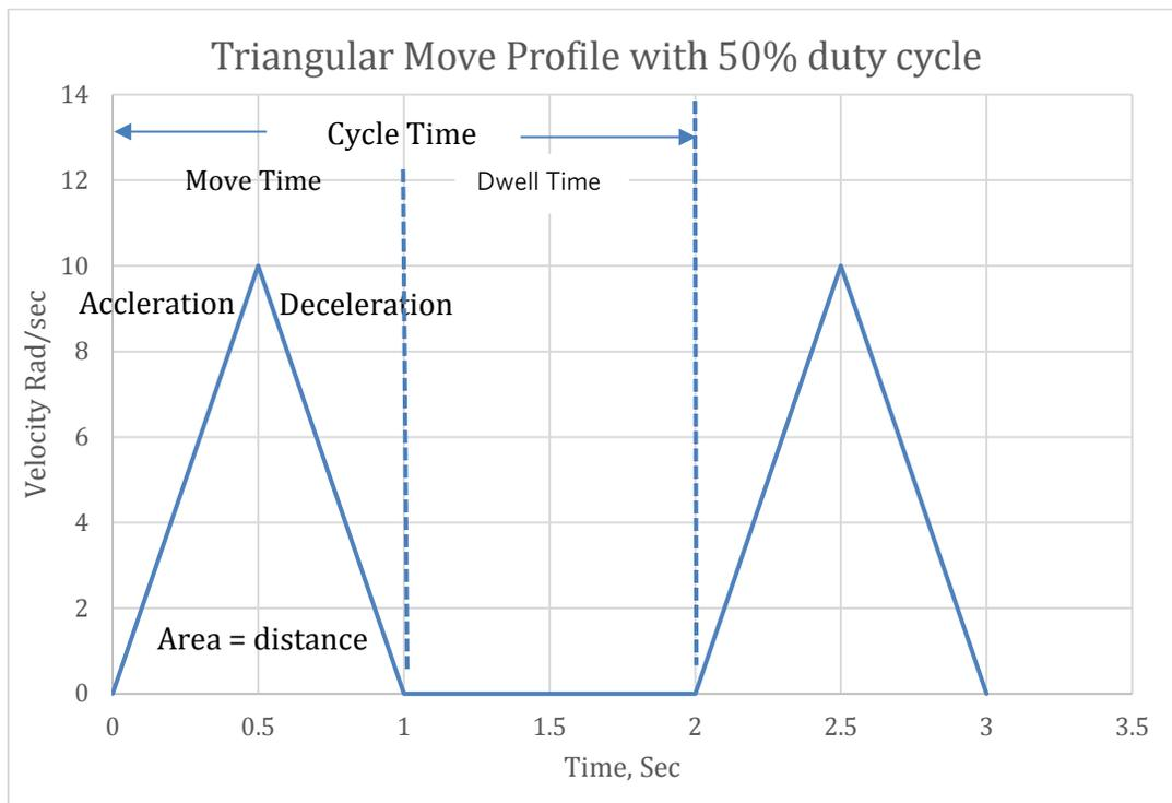
Figure 6 shows a repeated move with a 1 second dwell before the move repeats representing a 2 second cycle time for a 50% duty cycle.
