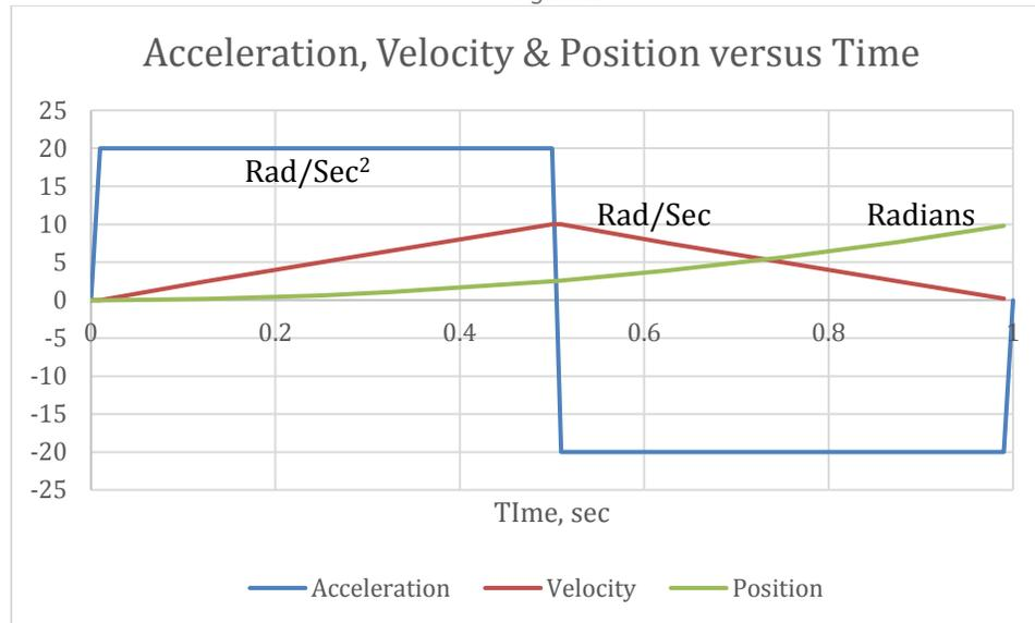
In Figure 2, the acceleration is constant at 20 rad/sec<sup>2</sup> and should represent a square wave. Position is shown in green. Note that halfway through the move in time is not half way in distance. This plot is meant to be a pictorial representation of all three motion states.
