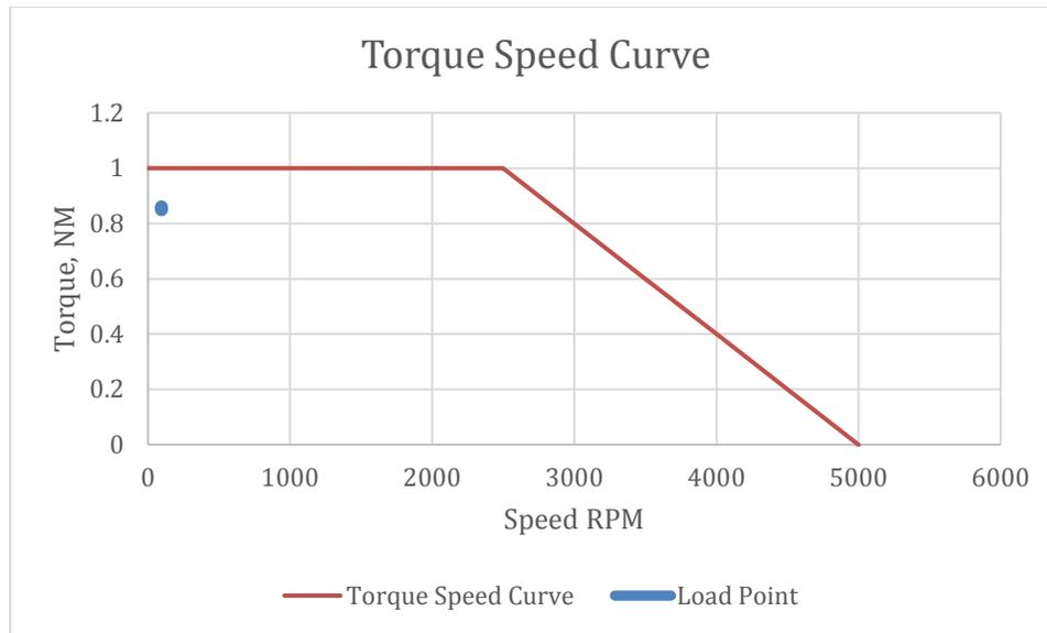
Figure 3 is a torque speed curve. Torque is on the Y axis and speed is on the X axis. The red data is the motor output defined by the input power available and the thermal limits (ambient temperature and maximum allowed motor winding temperature). Torque speed curves can be calculated for any motor using these electrical and thermal limits. Thermal limits can also be altered by changing the motor environment or adding passive or active cooling to the motor housing.
