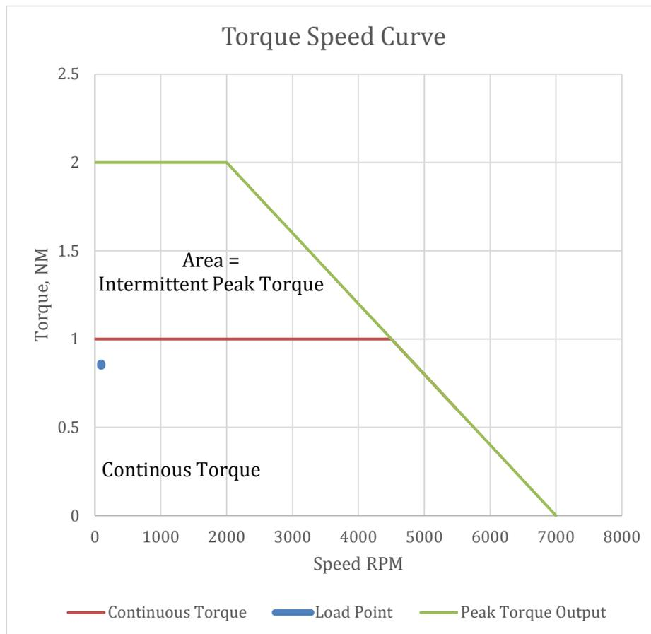
Figure 5 shows the same motor as Figure 4 operating at higher voltage. Higher voltage allows the motor to hold its torque points out to a higher speed before becoming voltage limited. Peak torque is held to 2000 rpm and maximum speed is now 7000 rpm.
